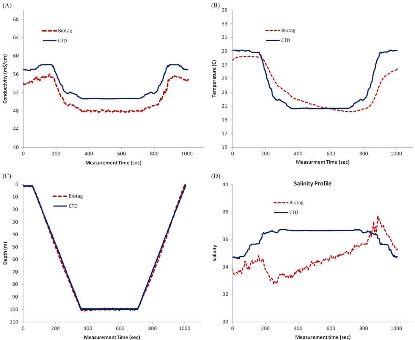
**Fig. 2.** Conductivity (a), temperature (b), depth (c) and salinity (d) profiles recorded in the Gulf of Mexico September 2011. The blue solid line represents measurements from the Sealogger CTD SBE 25 instrument and the red dotted line represents the biotag measurements.
