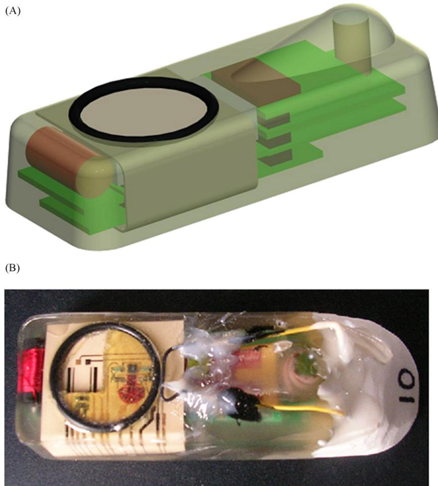
**Fig. 1.** (a) A schematic representation of the biotag showing the streamlined and smoothed contour along with the internal circuit board layout. The circuit boards were arranged in a multi-stack elongated configuration. (b) A photo of a packaged biotag with the front end tapered for increased hydrodynamic effect. Visible within the O-ring is the CTD sensors encapsulated in the soft-gel material.
